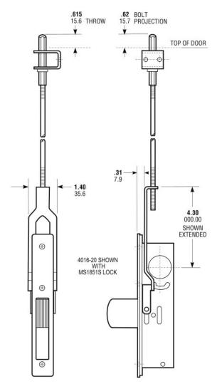
INSTALL ADAPTOR ARM TO LOCK FROM TOP WITH BOLT RETRACTED AS SHOWN. INSTALL PIN THROUGH SLOTS IN LOCK SIDE PLATES, PASSING THROUGH HOLES IN BOTH SIDES OF THE ADAPTOR ARM.
